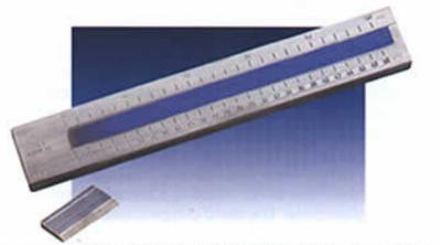
Same construction and use as the Hegman gauges (no. 2020, page 14), these grindometers are graduated in  $\mu m$ , with an accuracy of  $\pm$  1  $\mu m$ .
